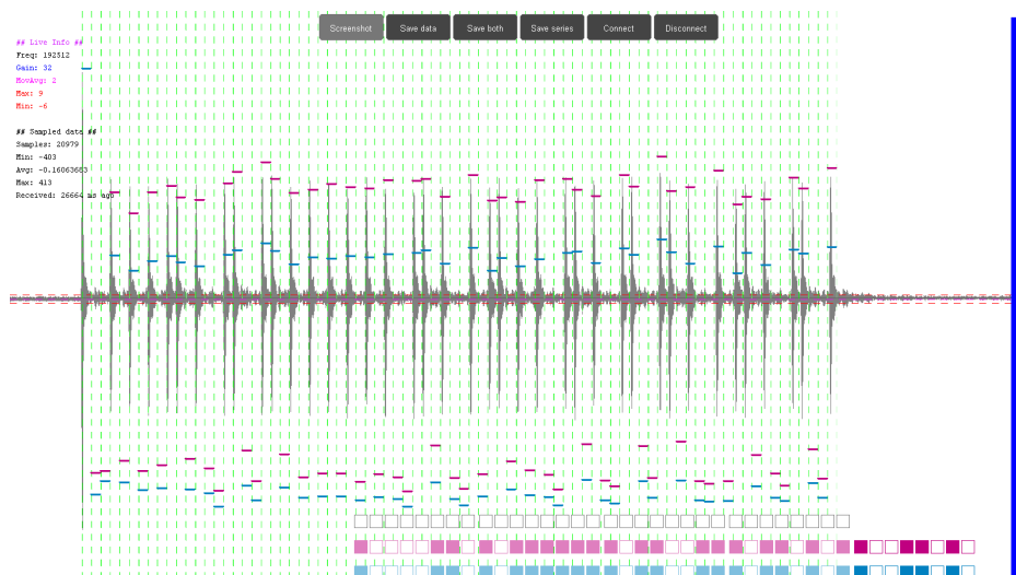
Figure 4: Successful transmission of 32 bits plus 8 bits CRC at 500 bits per second
